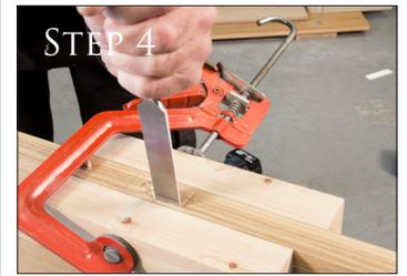
Depending on the thickness of your door it may be worth bracing the door with some scrap wood and a G clamp as the latch faceplate might be very close to the edge of the door.
